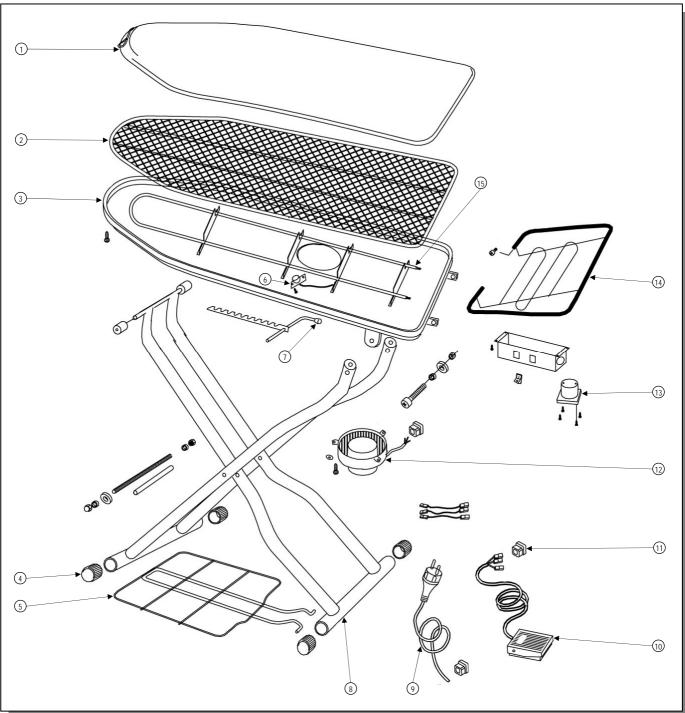
The machine is composed of the following main components: Exploded drawing of the table SUN
