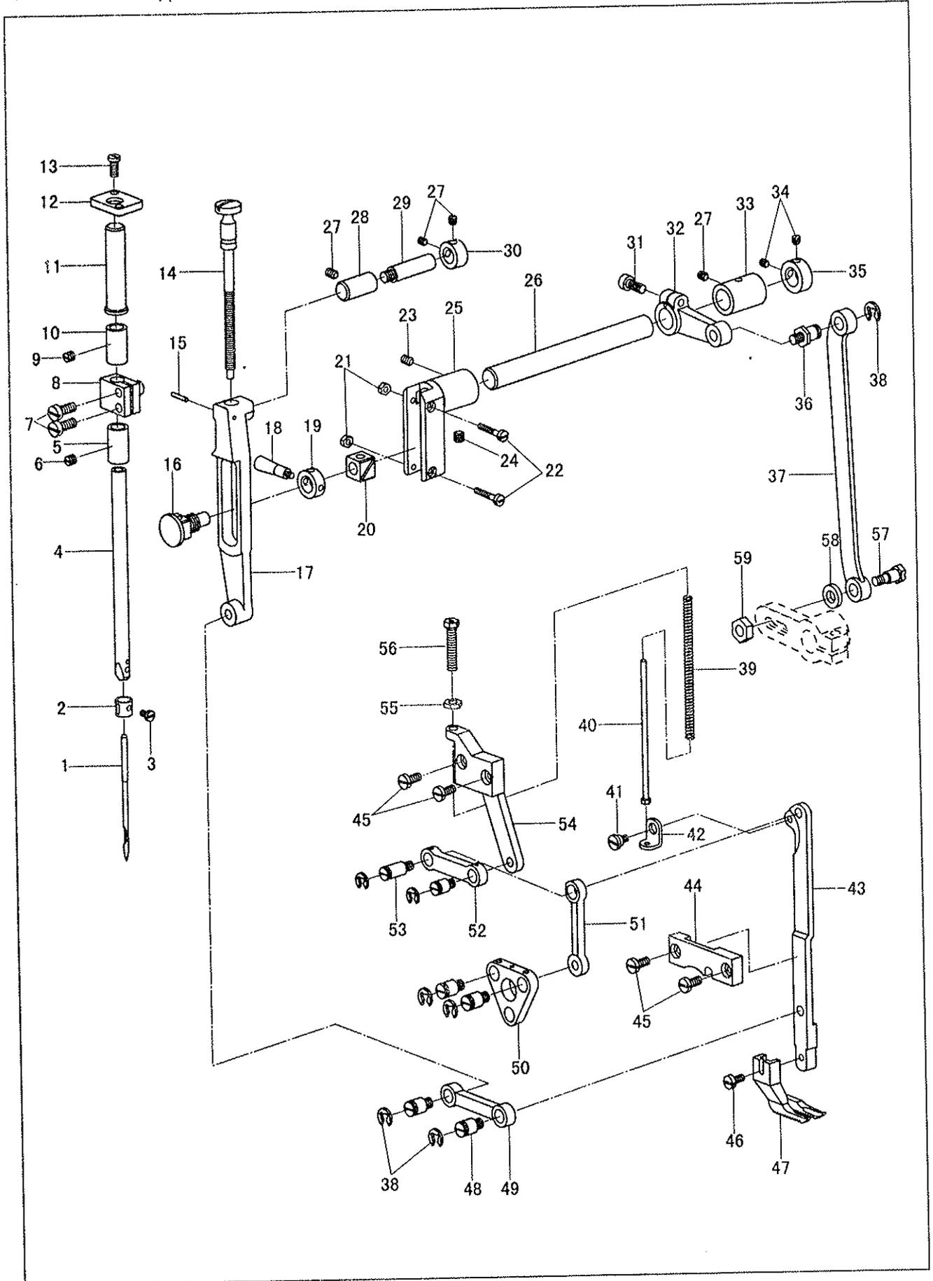
4. Needle bar and upper feed components(TW1-273)
