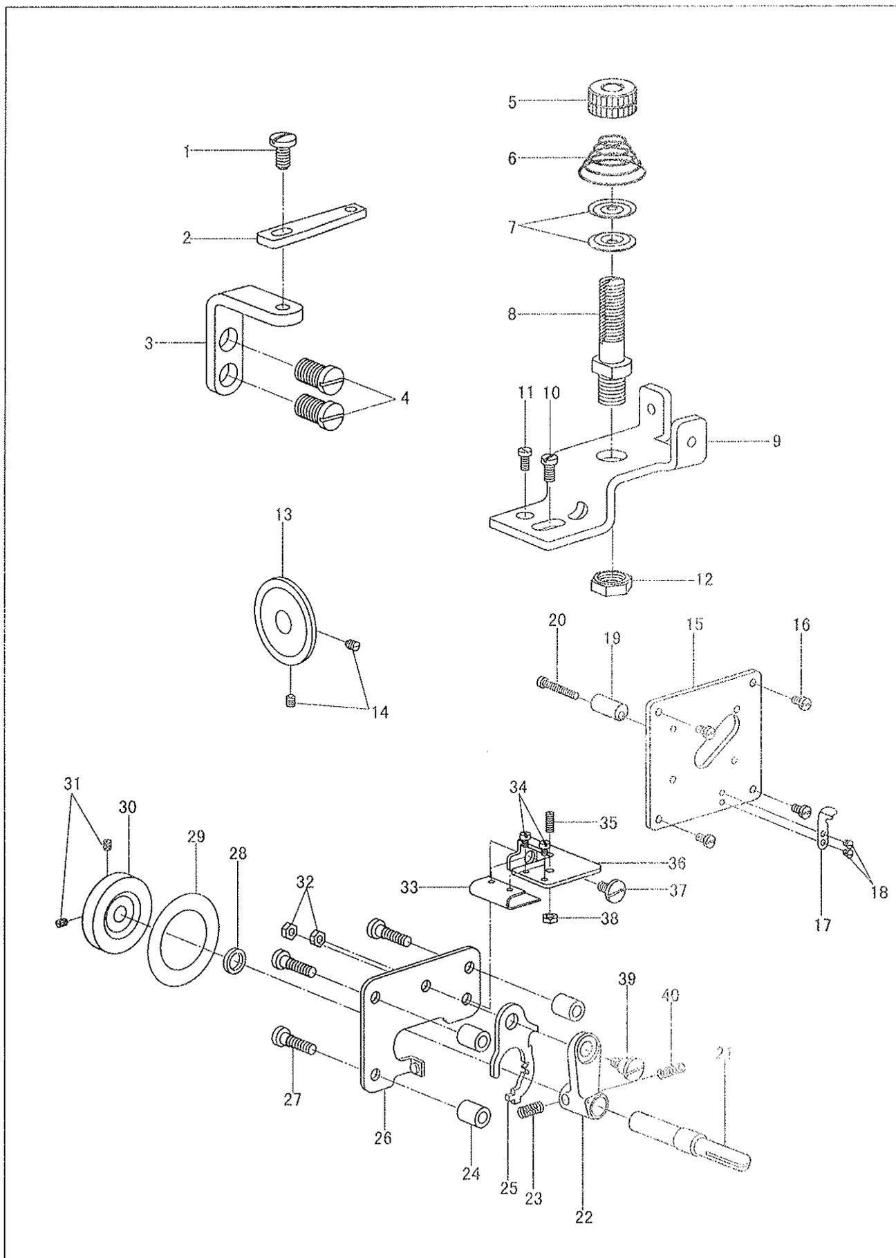
10. Bobbin thread winding components
