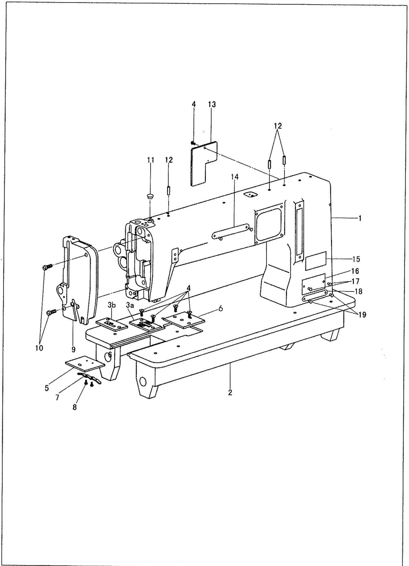
1. Machine casting components
