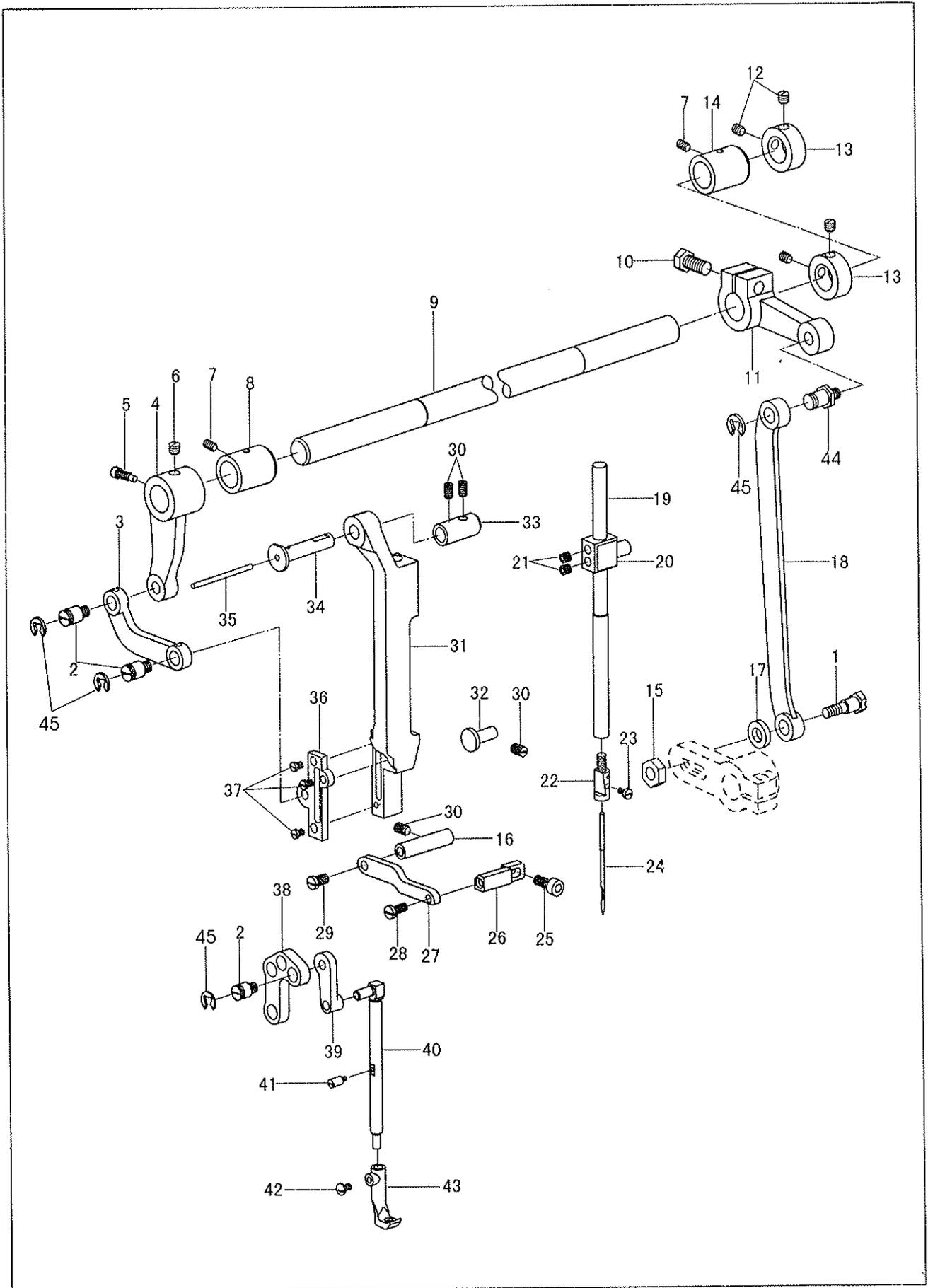
3. Needle bar and upper feed components(TW1-243)
